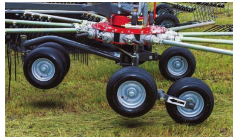
Patented, fully cardanic rotor suspension
