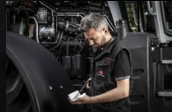
Front axle and slim waist bonnet design make oil dipstick and filter access easy.
