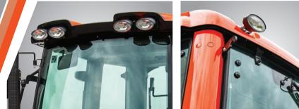
**Front and Rear Work Lights** Adjustable front and rear work light allow the operator to maneuver safely in low light conditions.
