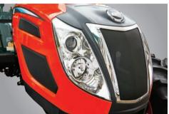
Projection Lamp Newly designed headlights allow the operator to see and work safely even in low light condition.
