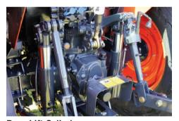
**Rear Lift Cylinders** Heavy rear linkage and 2 large assist cylinders with a lift capacity of 3630kg at 24" behind ball ends.
