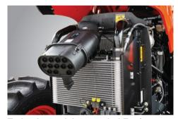
**Turbocharged, Intercooled Engine** The turbocharged engine with Air to Air Intercooler ensures the PX Series has the power the operator
