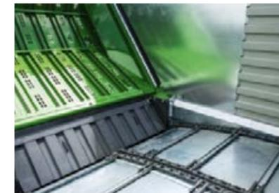
To protect the rotor against corrosion and contamination when working with maize, the Fendt Tigo has a maize channel cover that can be fitted quickly and without tools.
