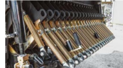
Use the FlexSharp knife sharpener to sharpen the knives without removing them.
