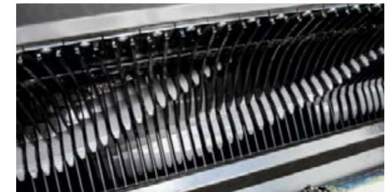
With a diameter of 800 mm and 7 spiral tine rows made of Hardox steel, the rotor is equipped on both sides with large spherical roller bearings.
