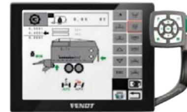
Control the bulkhead and the cutter unit on your terminal. Even the pick-up and drawbar can be conveniently adjusted from here.
