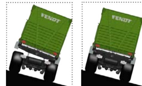
Without the automatic levelling control, the vehicle tilts downwards or to the side on slopes depending on the load and cornering speed (see Figure left). With the automatic levelling control from the FSC, the vehicle always stands parallel to the slope. The vehicle always adjusts to the best chassis height depending on the load (see Fig. right).
