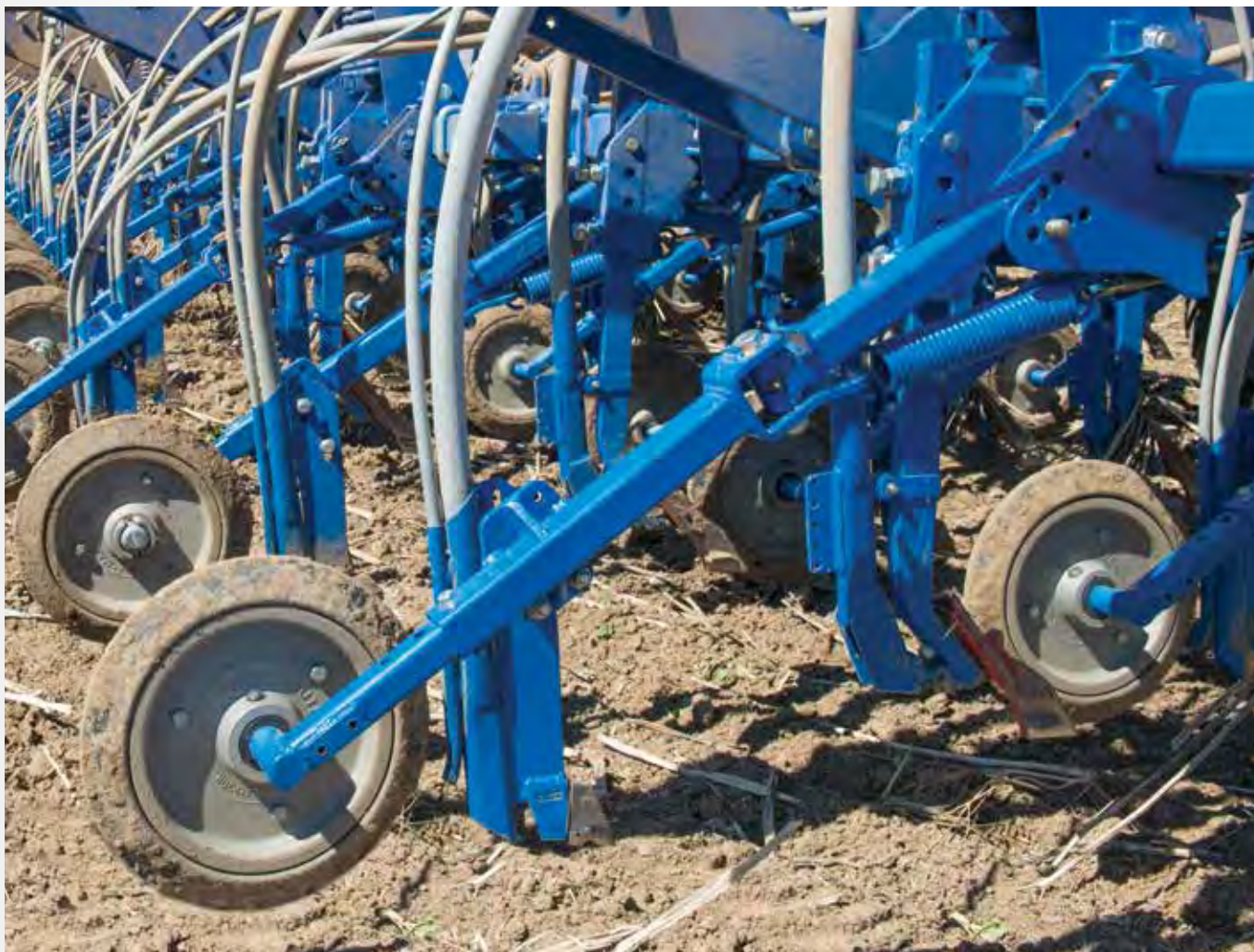
Optional seeding boot attached to press wheel provides better seed depth control. Mud scraper optional.
