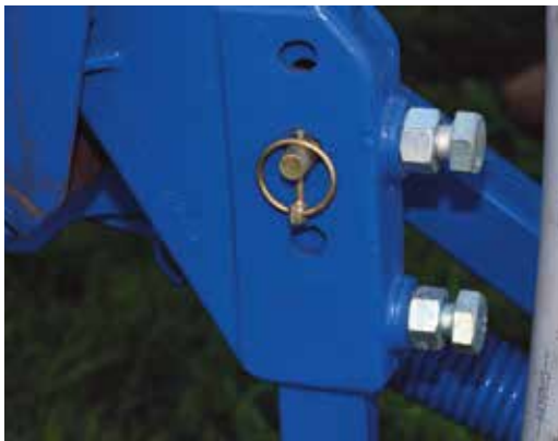
Depth adjustment in 12 mm increments.
