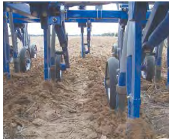
Trash clearance is exceptional with straight edge on tines, a clean underframe and minimum 800 mm between rows.
