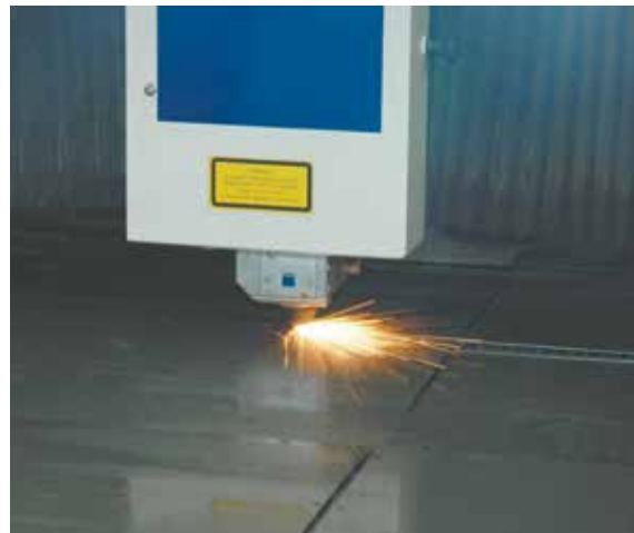
Laser cut parts are accurate to 0.1mm.
