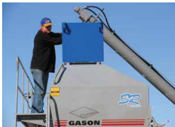
Offset bin openings on the 1860 series seeders allow operator to stand upright while filling.
