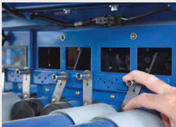
Meterwheel access windows on the SR meterbox removed.
