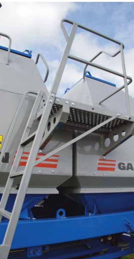
Offset bin openings on the 1860 series seeders allow operator to stand upright while filling.
