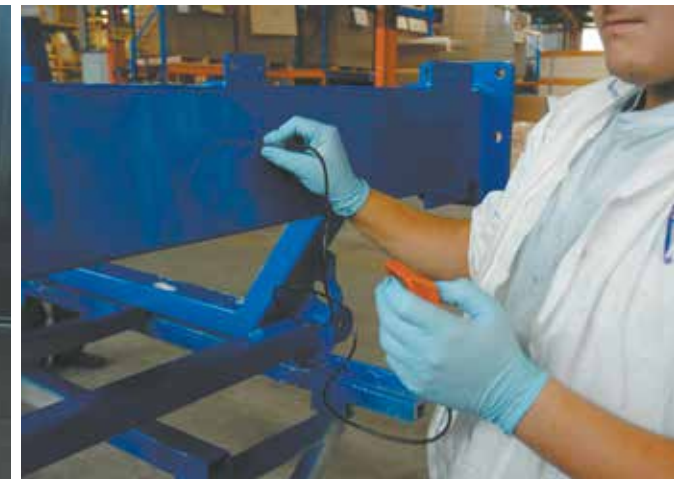
Paint depths are electronically checked.
