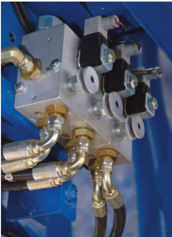
Manual override controls allow seeding to continue in the event of electronics failure.
