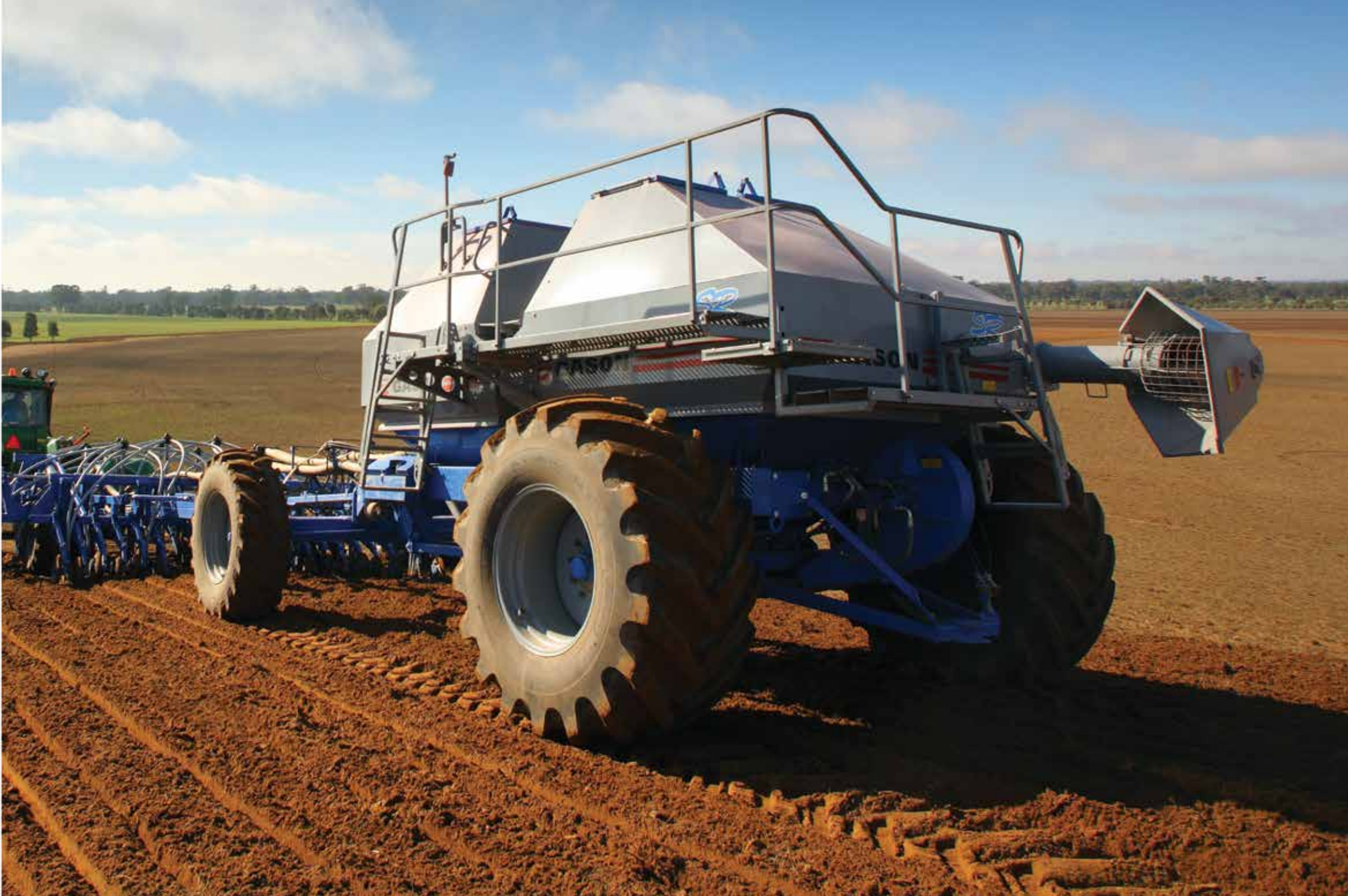
2120RT 3 bin VRT seeder with rear walkway option, rear hitch and auger fitted
