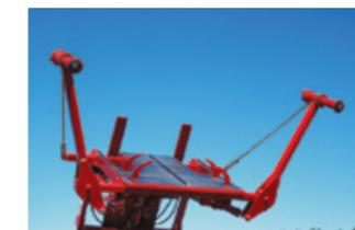
Grab hooks hold the first bale in place. Unique floating pipes on the alignment arms hold the second bale, to create the forward stair-step.
