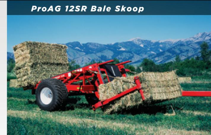
Automatic grab hooks hold the first bale in position, without dragging the bale, allowing the alignment arms to reopen to engage the second bale. The loader automatically rotates up as the two bales are squeezed. Bales can be picked in any orientation. The loader, alignment arms, and grab hooks are sequenced on one remote. Stair stepping the bales during loading aids in helping the bales slide back on the bed.
