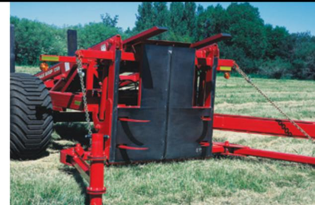
The Auto Align® system allows the operator to pick up bales in the same direction as the field was baled (12SR model shown).
