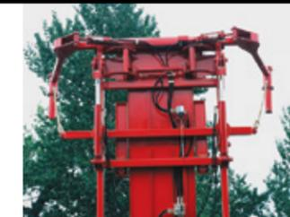
ProAG Bale Skoops feature a custom sequence valve and a 4-way valve to control the alignment arms, grab hooks and loader.
