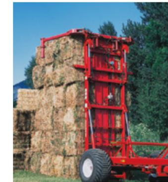
Once the bed is vertical, alignment arms are opened, and the 12SR is driven forward to remove the forks from under the stack.
