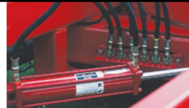
The hydraulic manifold (12SR shown) is located for easy access and servicing.
