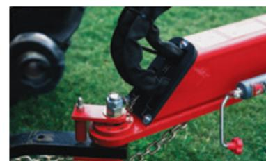
4x4 baler ball style hitch. Hydraulic hoses are sheathed and labeled for easy hook-up. Safety chain is included.
