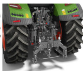
Quick-hitch frame with hydraulic opening of the tail arrester as standard
