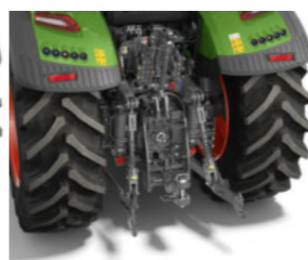
Rear power lift with quick arresters and rub blocks (AU, South Africa, Eastern Europe)
