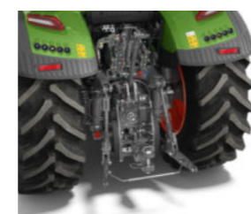
Rear power lift with ball ends and rub blocks
