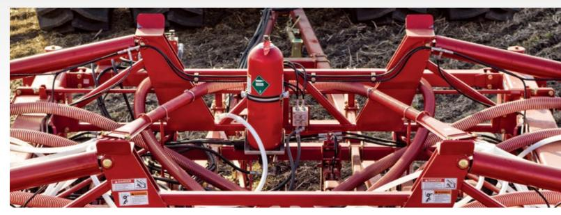
Pressure is maintained on the opener cylinders through a passive hydraulic system that uses a hydraulic accumulator. This unique hydraulic accumulator system acts as a hydraulic cushion for the trips, and being a passive system, greatly reduces the demand on the tractor hydraulics compared to the continuous flow required by similar drills. By adding or subtracting oil from the accumulator circuit, through a tractor remote,
