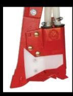
Optional mud guards reduce soil build-up on double-shoot openers. Optional air hose grommets for double-shoot openers prevent straw and debris from falling into the top of the opener ports.
