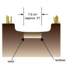
The **spread tip single-shoot opener** places a 3" (7.6 cm) wide ribbon of seed in each seed row. This opener cuts a smooth level seedbed resulting in very consistent seed placement and has been designed to minimize soil disturbance. The spread tip opener, with its high seed bed utilization is an excellent choice for farmers who apply low to moderate fertilizer rates with the seed.
