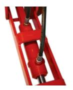
A double acting hydraulic cylinder raises and lowers the opener from working to transport position.
