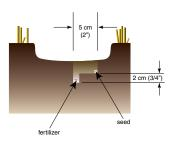
The **side band double-shoot opener** first places a distinct seed row 2" (5 cm) to the side of the knife followed by a fertilizer band which is placed directly behind the knife and 3/4" (2 cm) below the seedbed. This patented design results in outstanding fertilizer - seed separation and improved seed bed consistency by minimizing soil fracturing.
