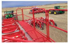
Filling of the tanks is made easier by designing the tank lids to be closer together. With the optional hydraulic assist the operator can use the wireless controller to position the spout on the auger/conveyor without moving the hopper from the unloading area or climbing down from the air cart. The lid design incorporates a gas cylinder to assist the operator when opening and closing the tanks. The handle
