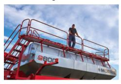
The walkway improves access to the tank lids. Handrails around the walkway platform and down the stairway provide excellent protection for a secure and safe work area. The walkway is positioned to allow the operator more room to work and avoid dust when filling the tanks.
