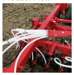
The patented flat fan divider heads maintain the smooth horizontal flow of product as it leaves the primary runs to the divide into each secondary run. This accurate and efficient air delivery system ensures that germination, growth and vigor are protected.
