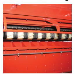
The time-proven spiral fluted metering wheel is the center of the metering system. The spiral flute provides a continuous flow of product into the air stream. The meter-bodies include single person operation of the inspection and calibration left side access doors. Calibration doors speed up calibrating time because the operator does not have to pick up parts from the ground. The 9800 and 91000 metering bodies accommodate up to 10 metering wheels.
