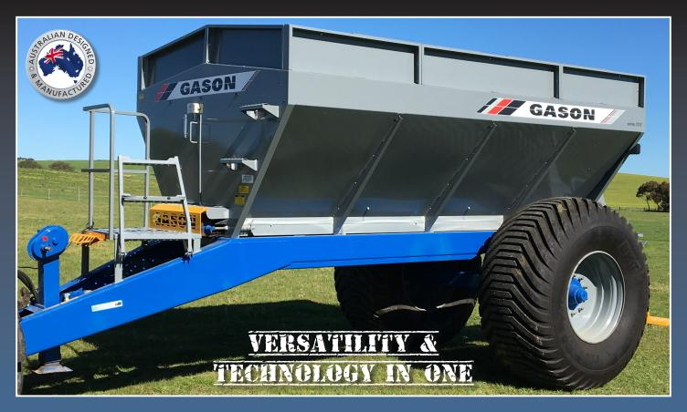
The new 9.4 and 12.8 tonne spreaders from Gason will spread up to 36m of pelletised fertiliser with the new widespread spinner discs which are the result of years of research and development at Gason. The system utilises a removable Widespread Centre Vee that provides increased flexibility when changing from different products such as lime, gypsum and urea.
