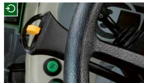
$\Box$  With the reverser lever, changing directions is easily done with the left hand.
