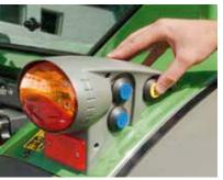
The Fendt 200 Vario has external controls for the linkage and rear PTO. Mount rear implements easily and save yourself unnecessary steps, for example, when filling the slurry tank.
