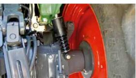
Thanks to the optional suspension, the Fendt 200 Vario cab is optimally supported on the rear axle. Shock loads and vibrations are absorbed by spring elements comprising shock absorbers and lateral stabilisers.
