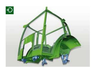
$\Box$  The Fendt 200 Vario can be fitted with cab suspension as an option. The cab rests on conical rubber bearings at the front, so that it is isolated from vibrations emanating from the tractor body. The helical spring shock absorber system at the rear of the cab reduces shock loads to a minimum.
