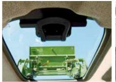
A hinged roof window provides additional ventilation and more upward visibility. The integrated roller shade provides protection against the sun.
