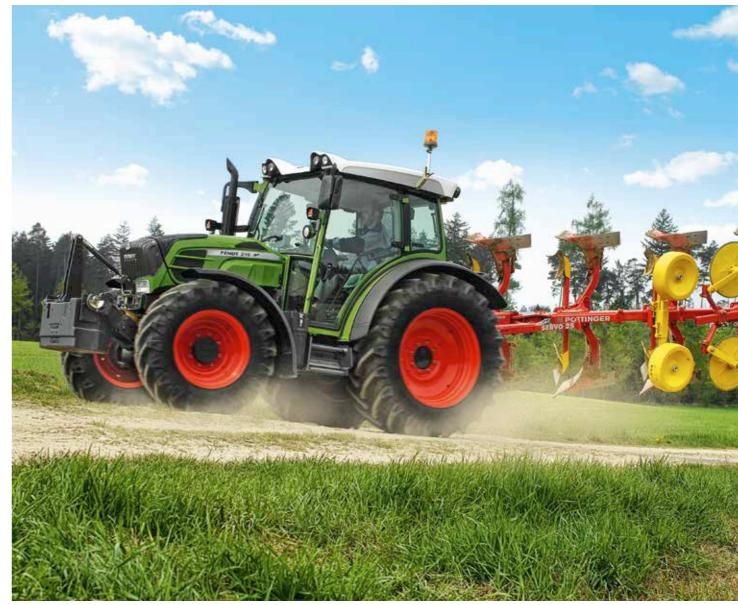
The front axle suspension has a total suspension travel of 90 mm along with a 20 degree swing angle. Self-levelling maintains suspension comfort, independent of payload. That guarantees safe braking and steering of the vehicle at all times.
