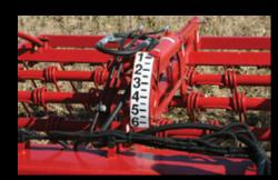
Hydraulic tine angle adjustment setting is conveniently visible from the tractor.
