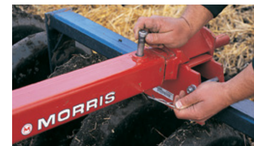
Universal Arm with quick detach pin for changing packers and harrows.
