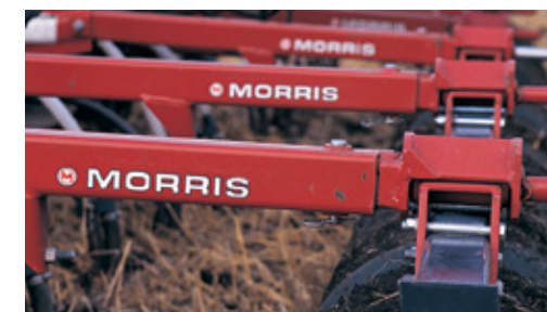
Universal Arm with quick detach pin for changing packers and harrows.
