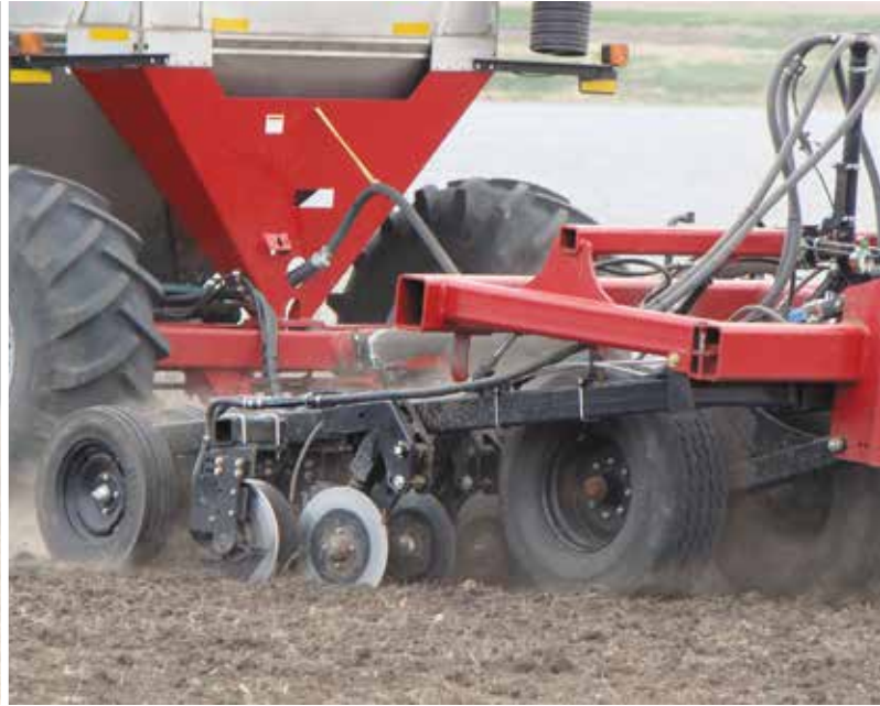
The discs lift and displace soil from the seed furrow and create enough loose dirt for the packer wheels to adequately pack.
