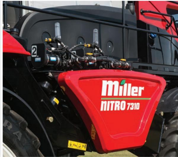
NEW redesigned adjustable chassis provides up to 78 inches of clearance. Its box steel construction uses 100,000-psi-yield high-strength steel for exceptional ruggedness and durability. A redesigned suspension system makes for a smooth ride.
