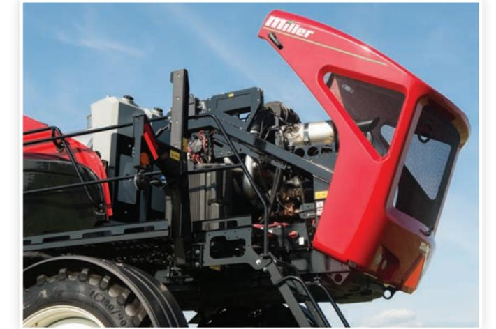
Engine and hydraulic service checkpoints are easy to access from the walkway by the engine compartment.
