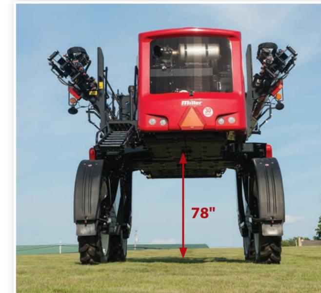
Highest ground clearance on the market! An industry leading 78 inches of ground clearance allows for late-stage application. Easily lower the overall height down to 153 inches (12.75 ft.) from the operator's seat for truck transport.
